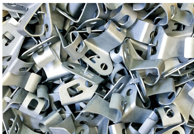
Blanked and formed aluminium automotive fasteners
