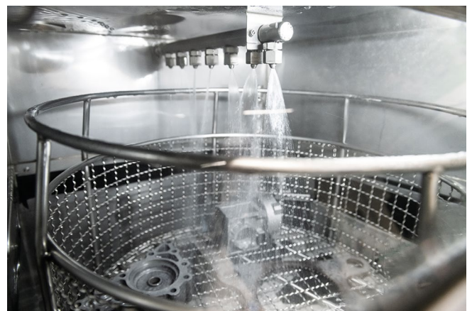
Cleaning process in an industrial washing machine
